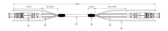
① LC UPC Connector ② Armored Tube ③ Ф7.0mm Outer Cable Jacket ④ Heat Shrink Tube ⑤ Strength Member
