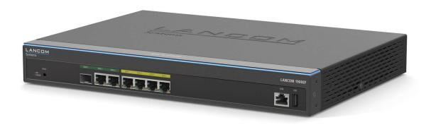
Multi-WAN VPN gateway for connection to high-speed fiber-optic networks and external modems—ideal for medium-sized VPN networking scenarios
